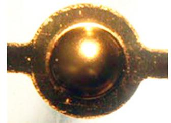
Goldeneye Ni (1.5  $\mu\text{m}$ ) + Techniphos 615 (0.5  $\mu\text{m}$ ) + Au-Ni (3  $\mu\text{in}$ )
