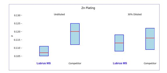
Left: Lubrus MS' friction coefficient performance vs a competitor's sealer on Zn plating.
