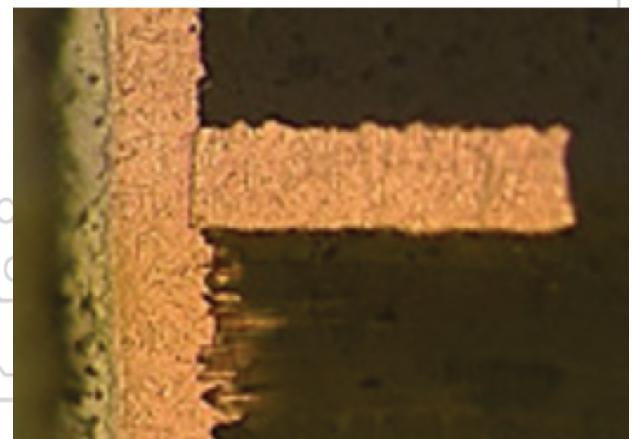
Excellent physical properties and grain structure between plated copper and inner layer.
