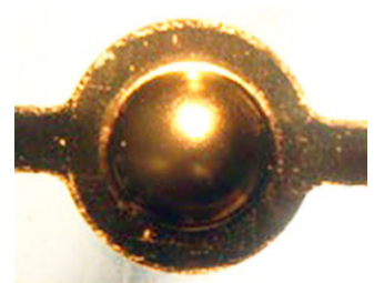
Goldeneye Ni (1.5 \mu\text{m} ) + Techniphos 615 (0.5 \mu\text{m} ) + Au-Ni (3 \mu\text{in} )
