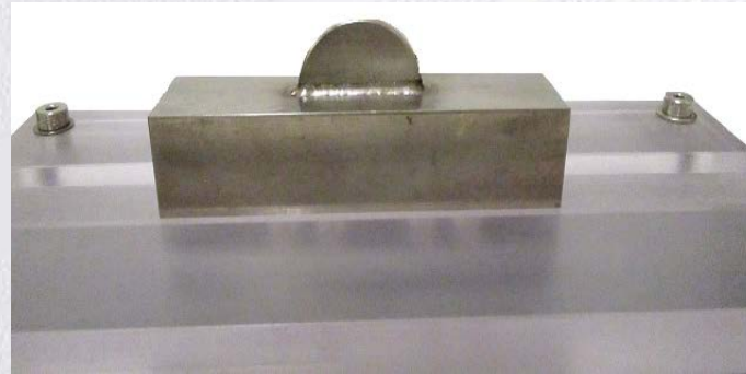
Picture 6: Weight on top of testing slide.
