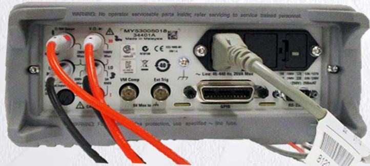
Picture 2: Ohm meter electrode hook up example.
