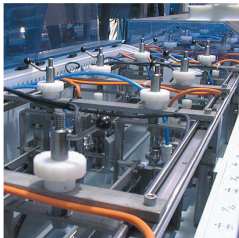
Controlled depth electropolishing station
